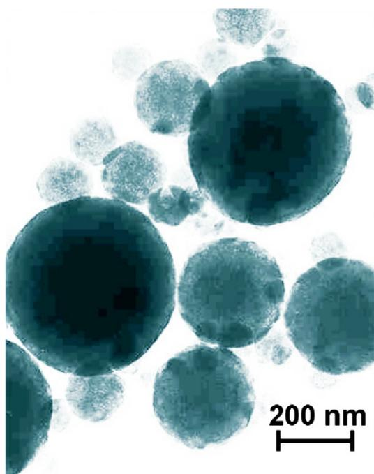
Fig. 1. TEM micrograph of sample Cr4, as prepared.
