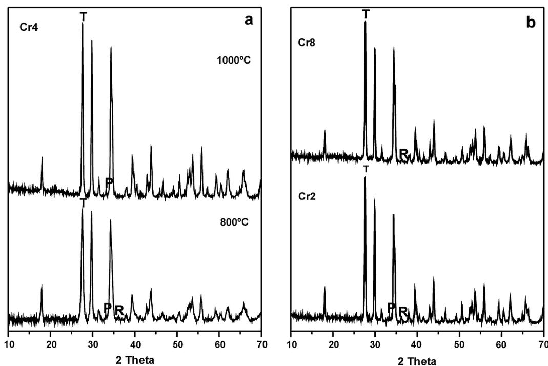
Fig. 5. X-ray diffraction patterns for sample Cr4 after heating at different temperatures (a) and for samples Cr2 and Cr8 calcined at 1000  $^{\circ}\text{C}$  (b). The most intense peaks of the titanite (T), rutile (R) and perovskite (P) crystalline phases labelled.
